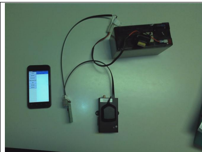
Picture 3. 12V supplied via RJ45/RJ12 splitter build-in into the BT1 module. BT1 module is powered by 3.3V supplied by the FLARM unit
