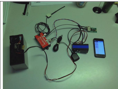
Picture 4. 12V is supplied to the RedBox FLARM. FLARM units supplies 3.3V to the BT1 unit and LX External Display. PT1 units is connected between the LX RedBox and the display unit. Apologies of the messy picture.
