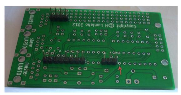
NOTE! Half of UART3 is used to make splitter for UART0, therefore pinheader to pin 13 is not used (red arrow).
