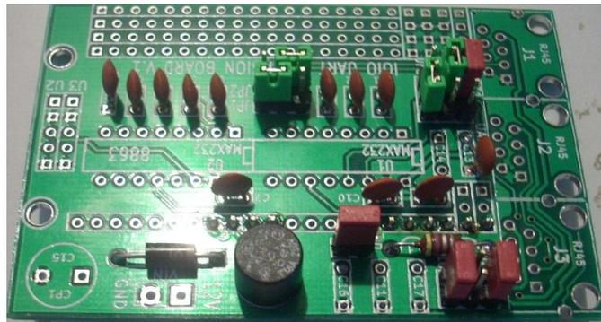
**Place and solder coil, fuse and diode.
