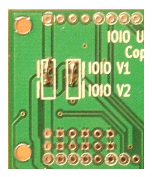
Solder connections made in image are for first generation IOIO card
