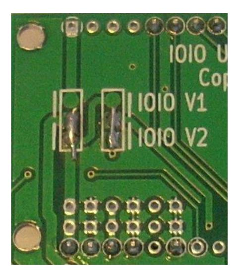
Solder connections made in image are for IOIO OTG card
